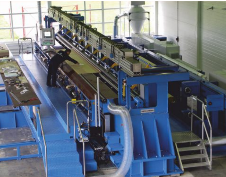
Fig. 16 Highly automated paper winding machine for 220 - 1150 kV bushings
