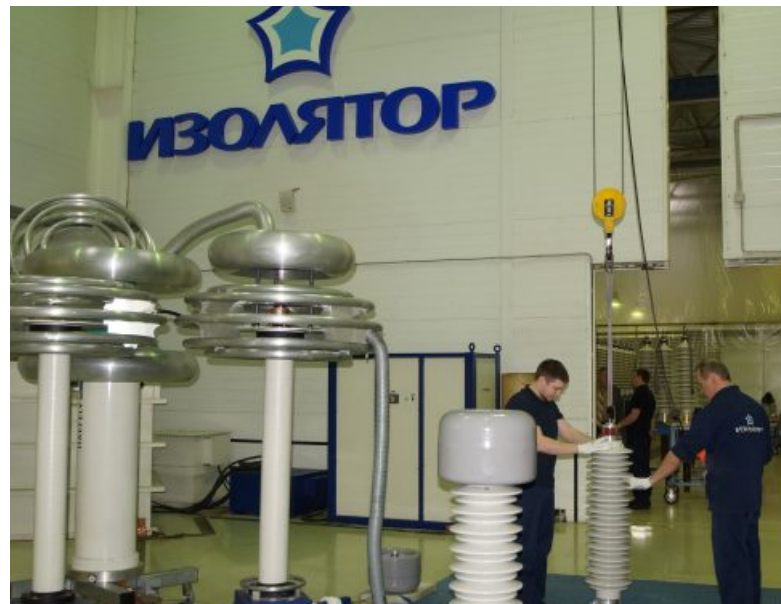
Fig. 23 Electrical tests of 110 kV bushings at Izolyator plant
