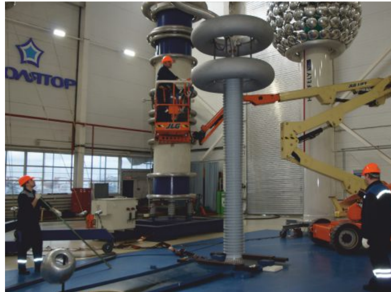
Fig. 22 220 - 1150 kV bushings test station at Izolyator plant
