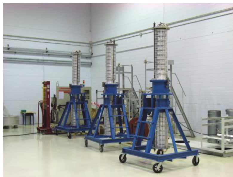
Fig. 21 Molding machines Hilger and Kern for manufacturing of external polymer insulation at Izolyator plant
