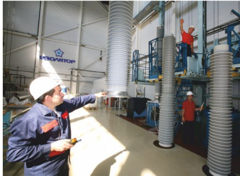
Fig. 19 500 kV and 330 kV bushings in assembly racks at Izolyator plant
