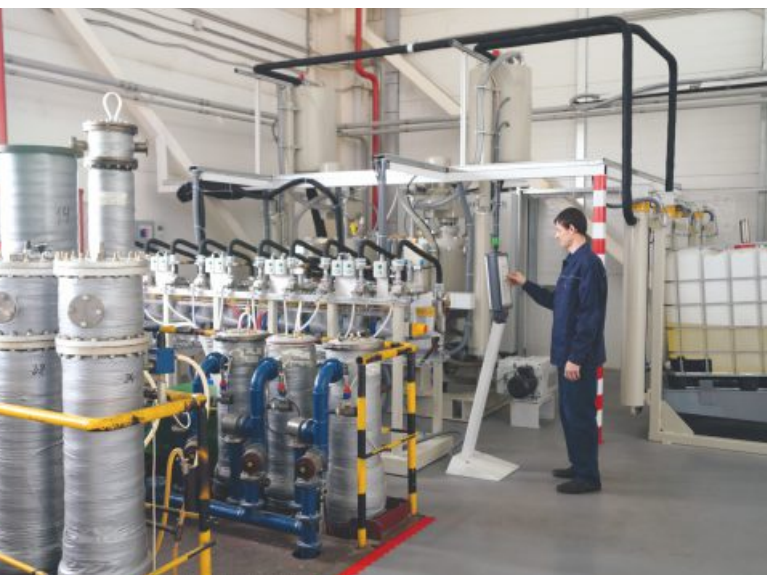
Fig. 17 Hubers machine for vacuum impregnation of insulation at Izolyator plant
