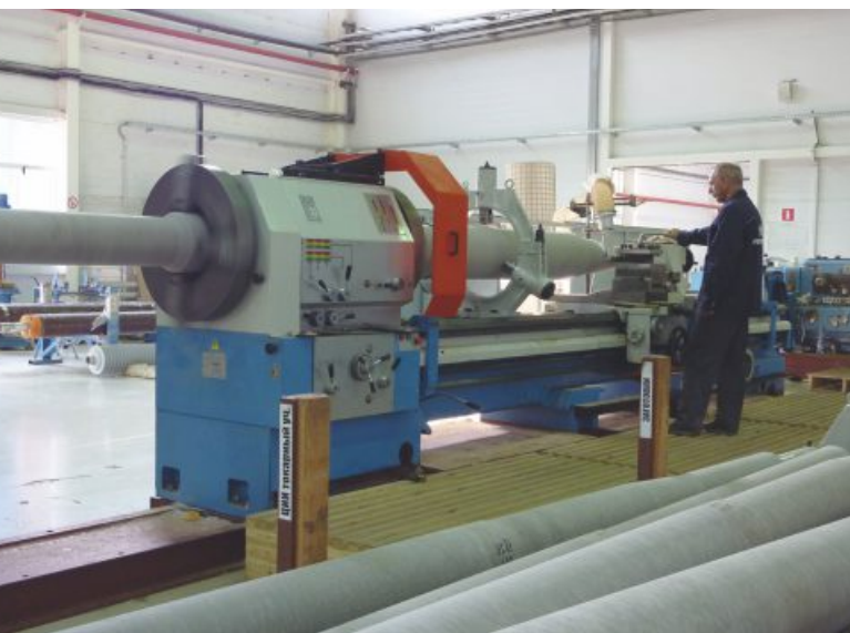
Fig. 18 Lathe turning of 500 kV RIP-insulation at Izolyator plant
